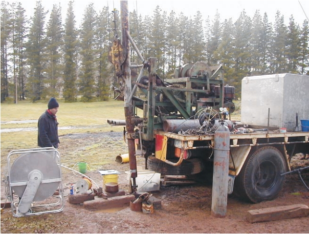
Fig. 3.9 Pump/packer set-up. (Photo 47940)
