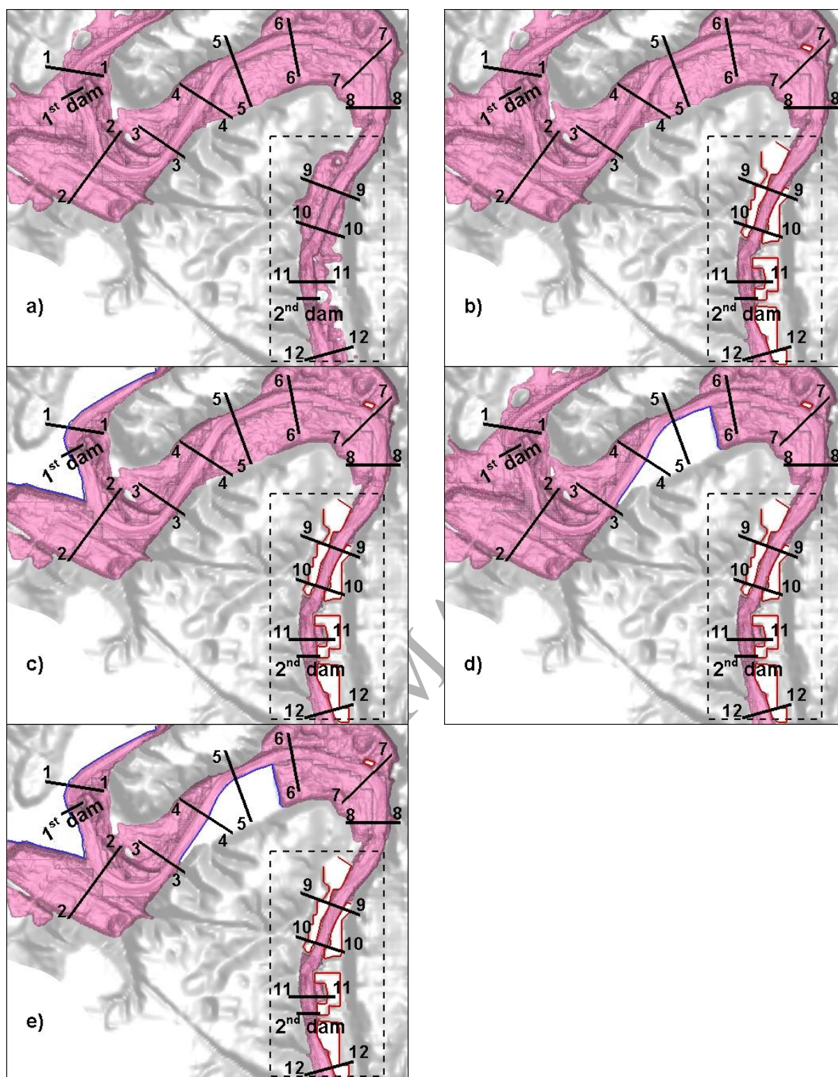
Figure 15. Flow in a 7-km long reach of the Iowa River. Flooded region predicted by the 3-D model at peak flood extent. a) base case; b) case Scenario 1; c) case Scenario 2; d) case Scenario 3; e) case Scenario 4.
